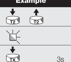
Note: If the memorization procedure has been successful the "radio LED" will flash slowly three times. If you need to memorize additional transmitters, repeat step 3 within the next 10 seconds. The memorization procedure will be terminated if no new codes are received within 10 seconds
