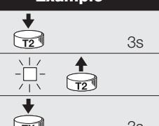
Note: If the memorization procedure has been successful the "radio LED" will flash three times. If you need to memorize additional transmitters, repeat step 3 within the next 10 seconds. The memorization procedure will be terminated if no new codes are received within 10 seconds.
